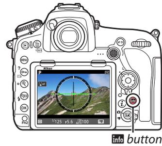
The virtual horizon shows roll and pitch based on information from the camera tilt sensors. If the camera is tilted neither left nor right, the roll reference line will turn green, while if the camera is tilted neither forward nor back, the pitch reference line will turn green and a dot will appear in the center of the display. Each of the divisions in the gauge around the circumference of the display is equivalent to 5°.
